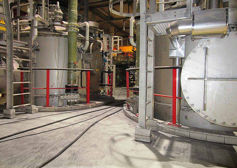
State-of-the-art process gas cleaning in the facility used to recover precious metals from anode slimes
